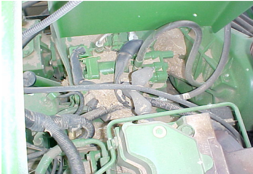
Figure 5. Harvester engine compartment with debris accumulation
